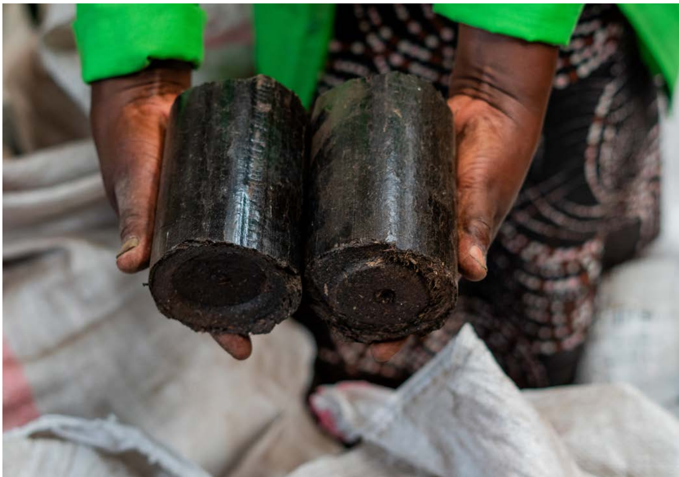
Briquettes made from bagasse at Sony Sugar Company. The briquettes are used as an energy efficient biofuel.
